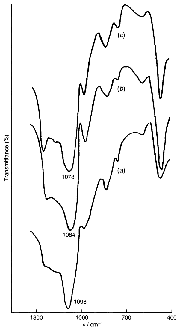
Fig. 1 Framework IR spectra of Si-MCM-41 (a), Sn-MCM-41(83) (b) and Sn-MCM-41(178) (c)
